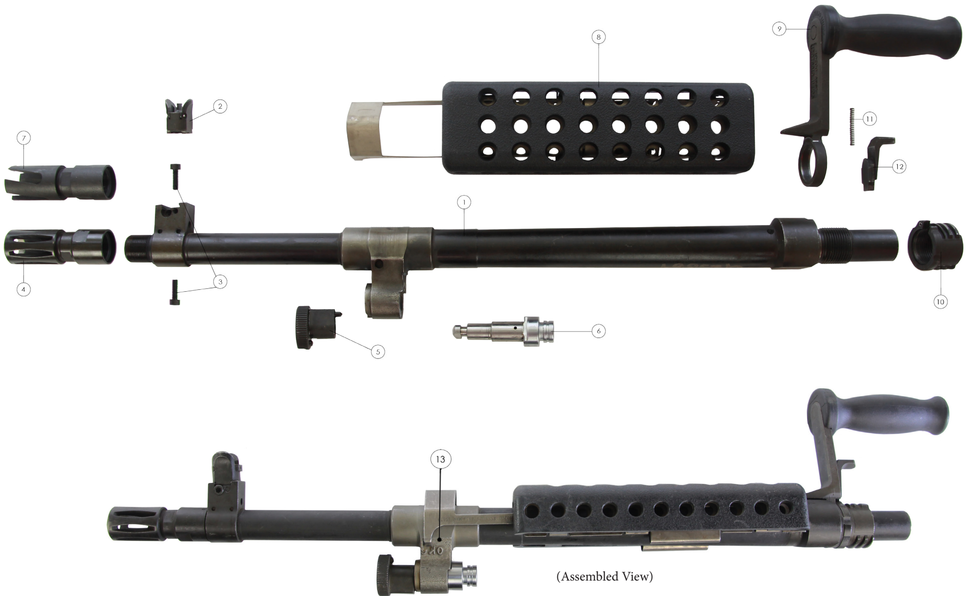
FIGURE 11. BARREL ASSEMBLY FOR CONFIGURATIONS 240B, 240D, 240G, 240H AND 240N
